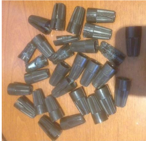
Figure F2 – Non-Petroleum based inhibitor failures
